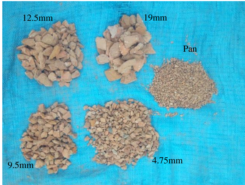
Figure 3.6 Crushed clay bricks retained on different sieve sizes
