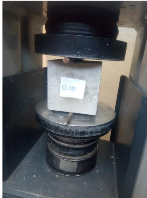
Figure 3.18 Set up for concrete specimen in compression machine for splitting Then the maximum depth of penetration is visually observed, marked and the maximum value for depth of penetration was measured and recorded to the nearest millimeters.
