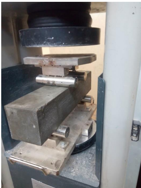
Figure 3.16 Two point loading setup for flexure test
