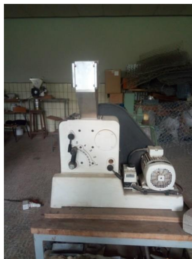
Figure 3.5 Jaw crusher used to crush clay bricks
