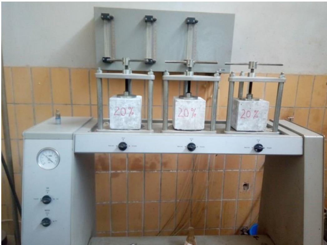
Figure 3.17 Concrete specimens setup on water penetration test apparatus
