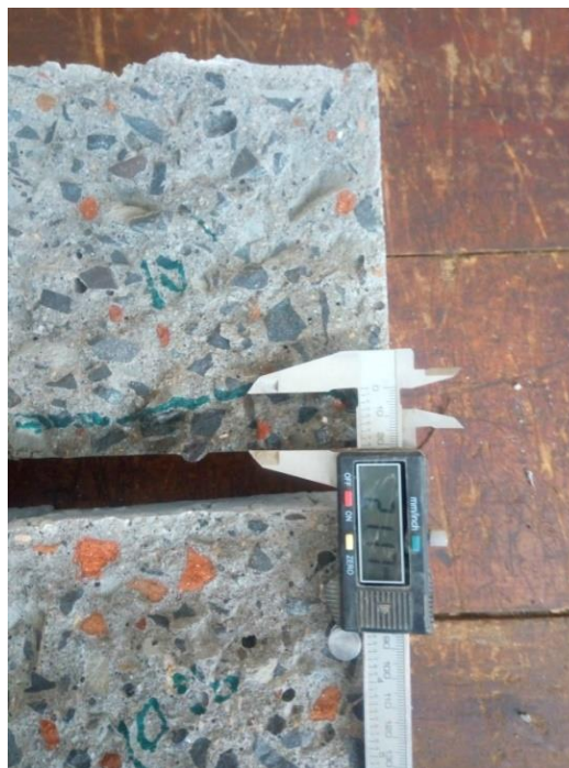
Figure 3.19 Measuring maximum water penetration depth from split concrete specimen
