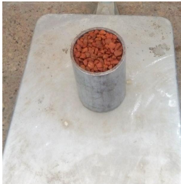
Figure 3.7 CCB aggregate tamped in cylindrical measure
