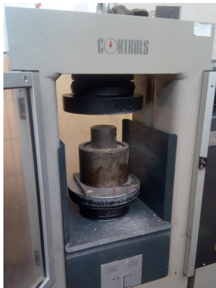
Figure 3.9 Cylinder setup in the compression test machine
