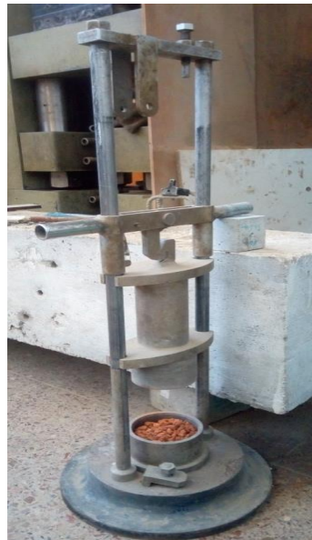
Figure 3.11 Set up of aggregate impact value testing apparatus
