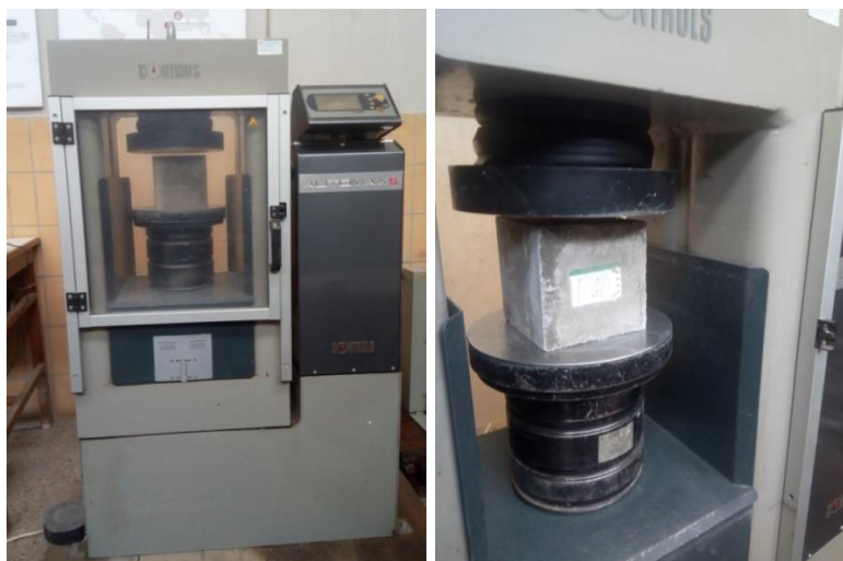
Figure 3.15 Cube specimen in compression test machine
