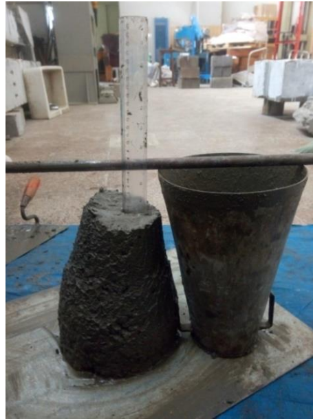
Figure 3.14 Slump cone test for the control mix (R)
