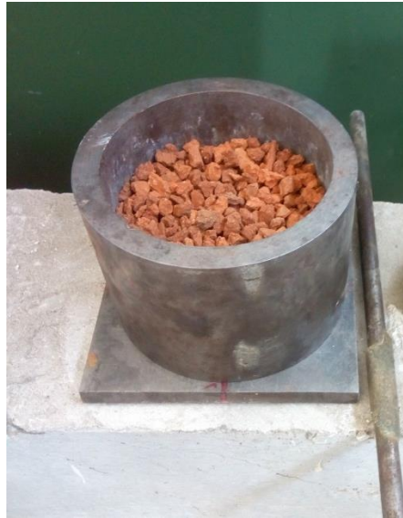
Figure 3.8 CCB aggregate tamped in open ended cylinder
