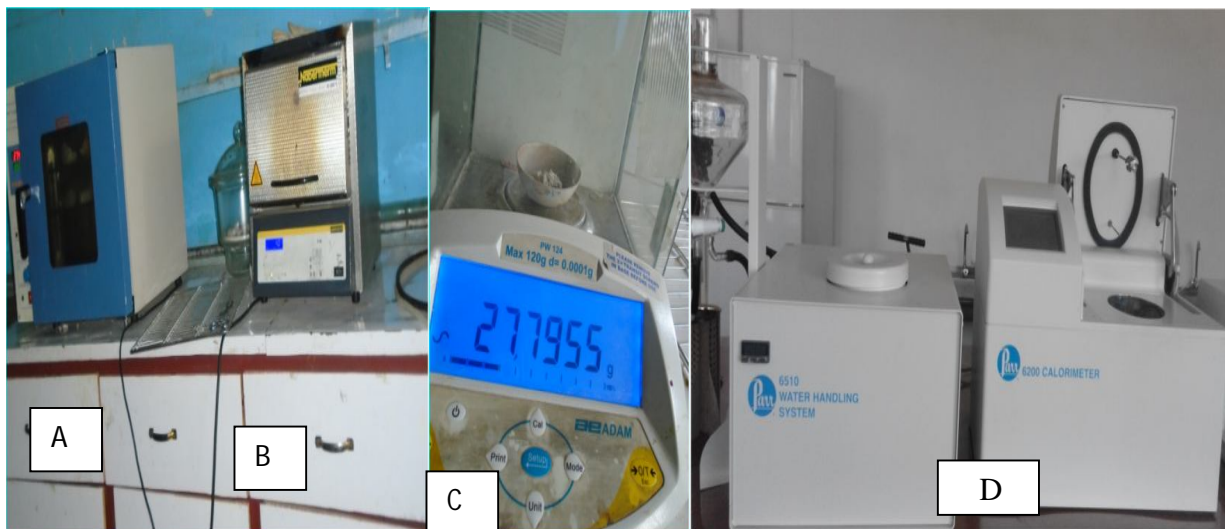
Figure 3.6: A; oven, B; furnace, C; Analytical balance, D; Oxygen bomb calorimeter
