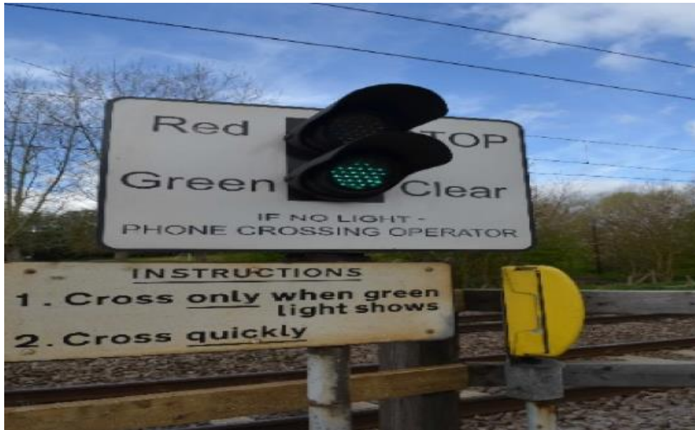
Figure 3-5: Miniature warning lights showing it is safe to cross[51]
