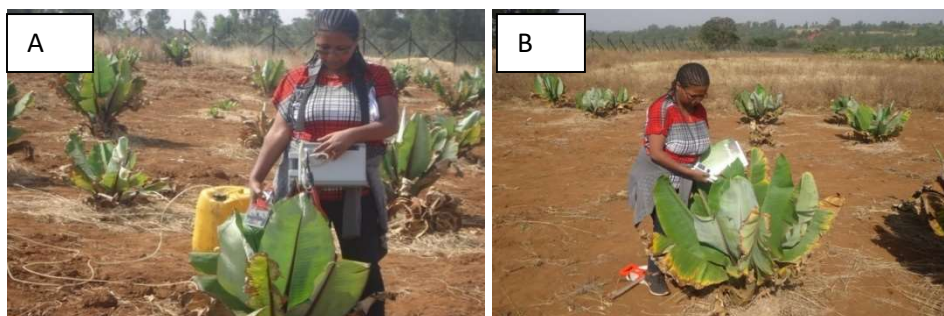
Figure 3. 10. Measurements of gas exchange parameters using LCPro+ (A) and Measurements of Chlorophyll content using SPAD-502 on the 3rd leaf (B)
