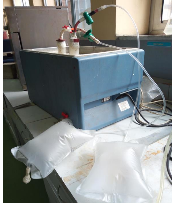
Figure C.5 Laboratory scale Anaerobic digestion setup
