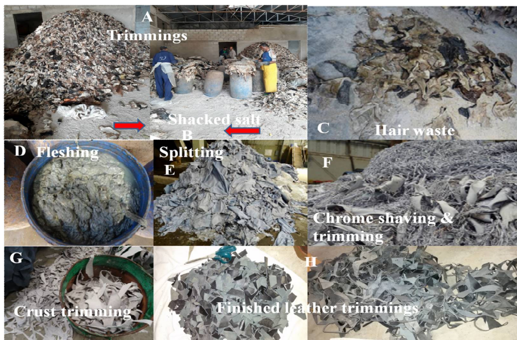
Figure 16: Solid leather wastes A, B & H photos taken during study; C, D, E, F & G photos from (Cristina, 2018)
