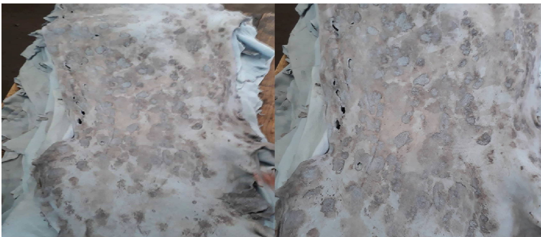
Figure 11: Putrefaction damage: (Picture taken at colba tannery during the study period in February, 2018).
