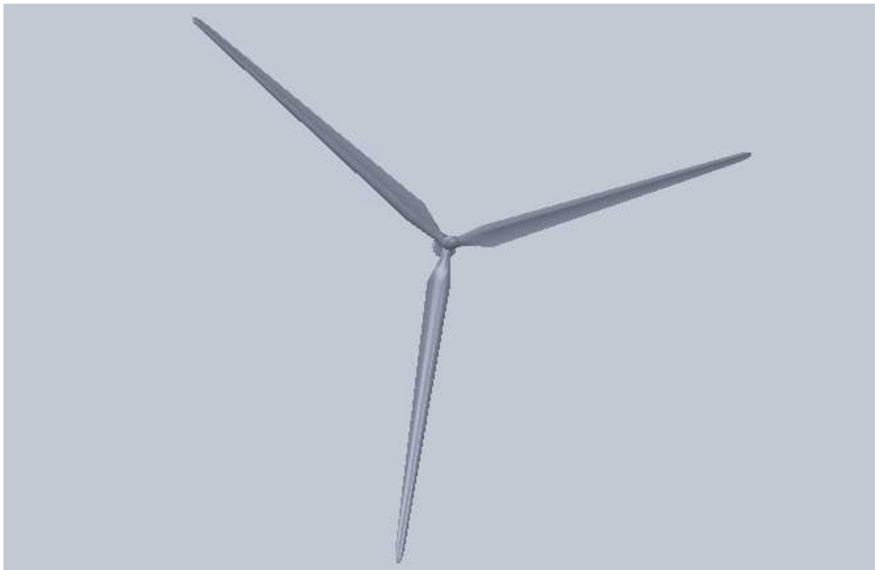
Figure 4.6 Three blades 3D solid model of the design blade by SOLIDWORK Model.
