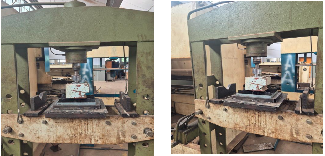
Figure 18 curing process of the laminates
