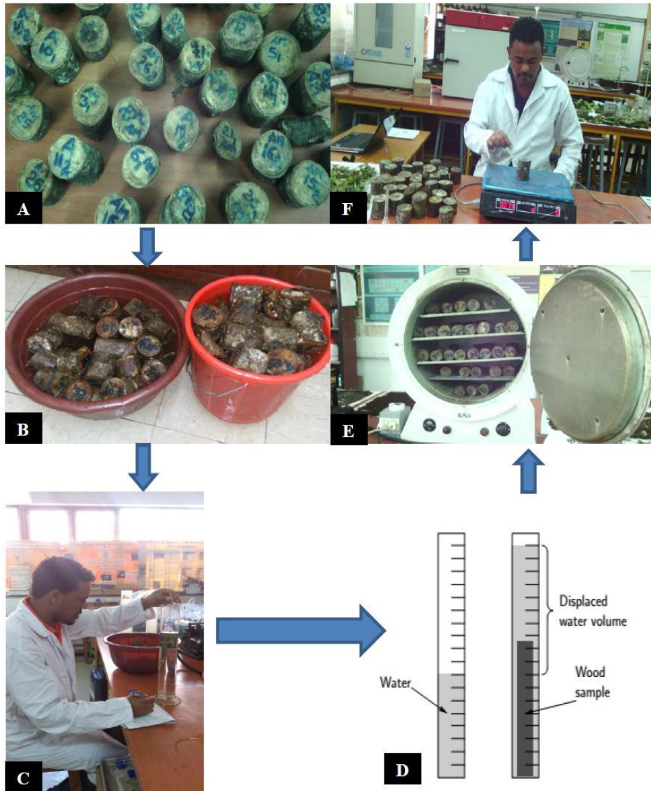
Figure 12. Procedures showing wood density determination of a typical tree species at Ecophysiology laboratory, AAU. A) collecting wood discs to laboratory, B) Rehydrating them, C & D) Measuring volume of discs, E) Oven-drying them , F) Measuring oven dry weight of discs.
