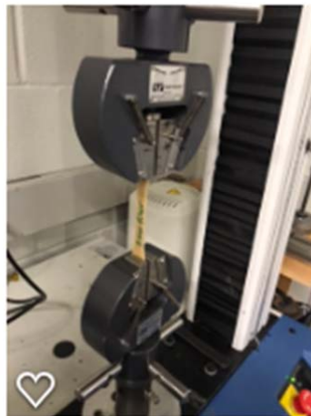
Figure 3-2-24 Instron™ Tensile Testing Machine for Determining Young's Modulus and Strength of the Test Specimen
