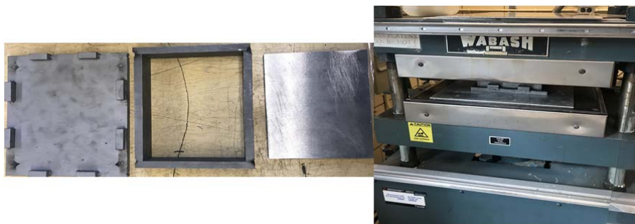
Figure 3-2-21 Mold Release Agent Mold Plate And Compression Molding Machine Used For the Preparation of Sample Plates.
