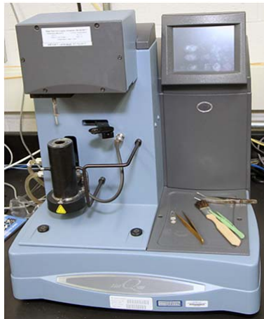
Figure 3-2-28 TGA Testing Machine Used To Test The Thermal Effect Analysis
