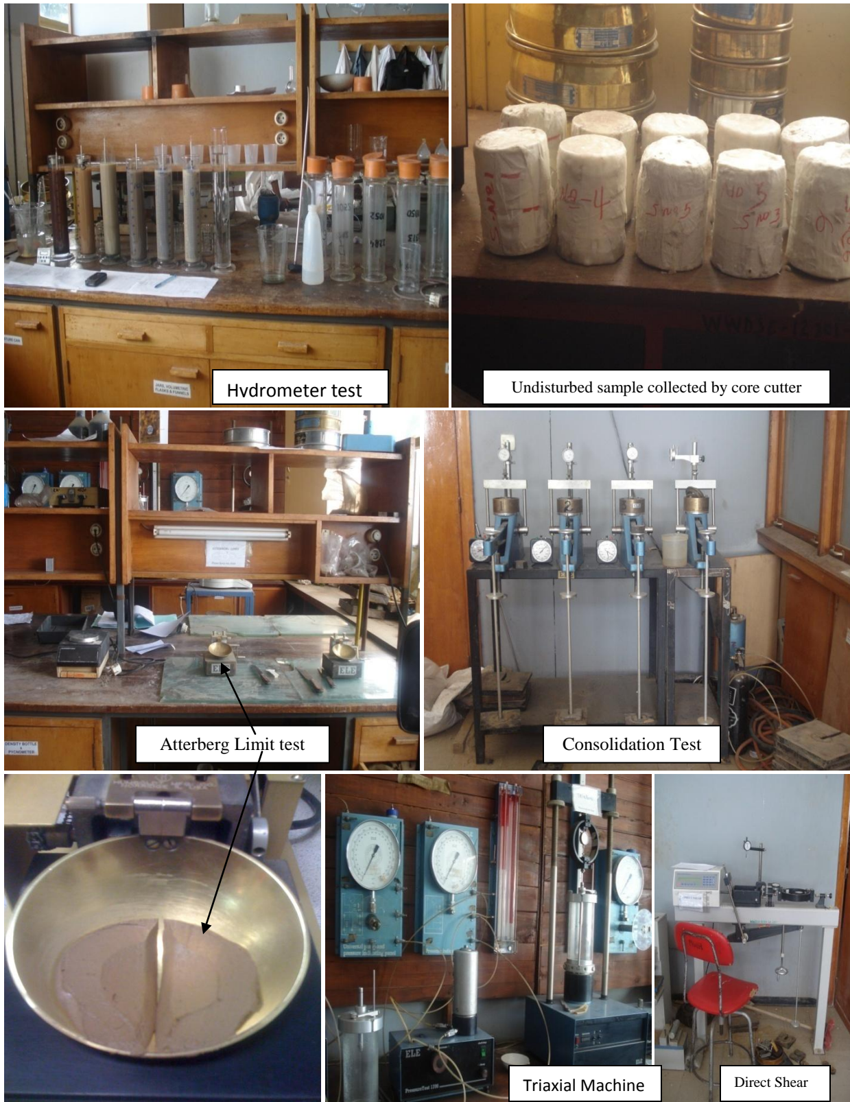
Plate 4: Some of laboratory test instruments used during the research study
