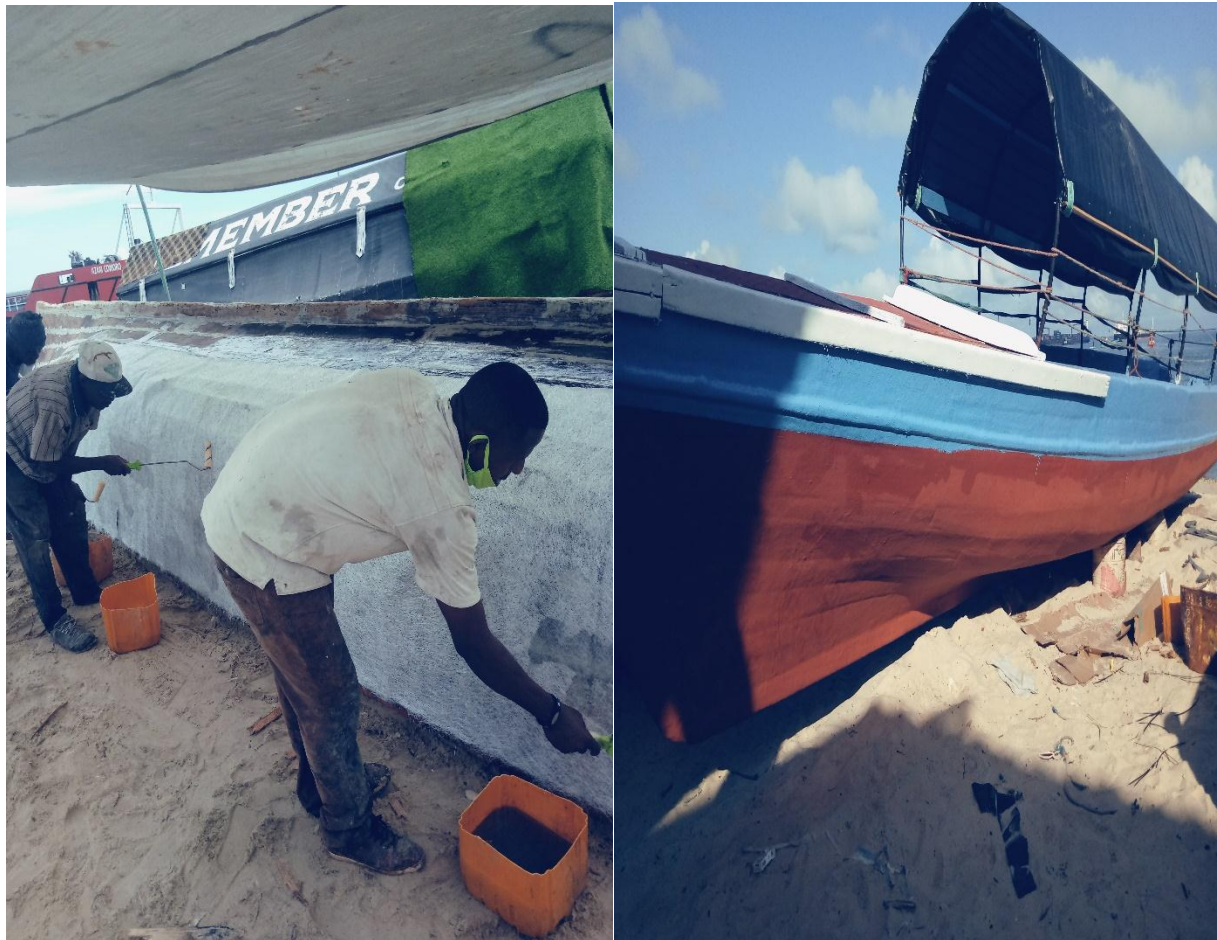
Plate 8: The process of carrying out Fiber net technique in a wooden boat.
