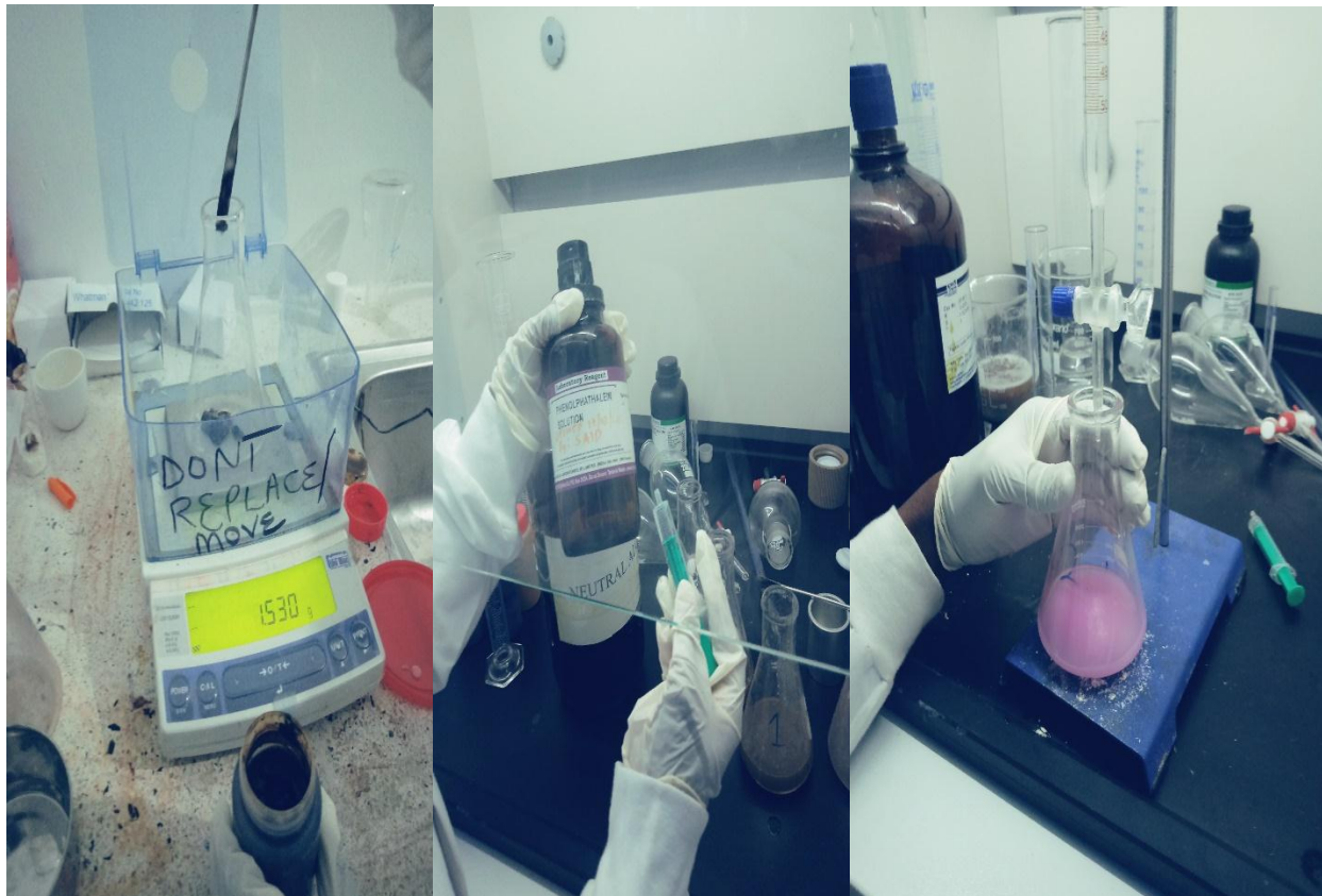
Plate 4: Determination of the acid value of the shark liver oil. (Photo credit: Suleiman Ally, 2021).
