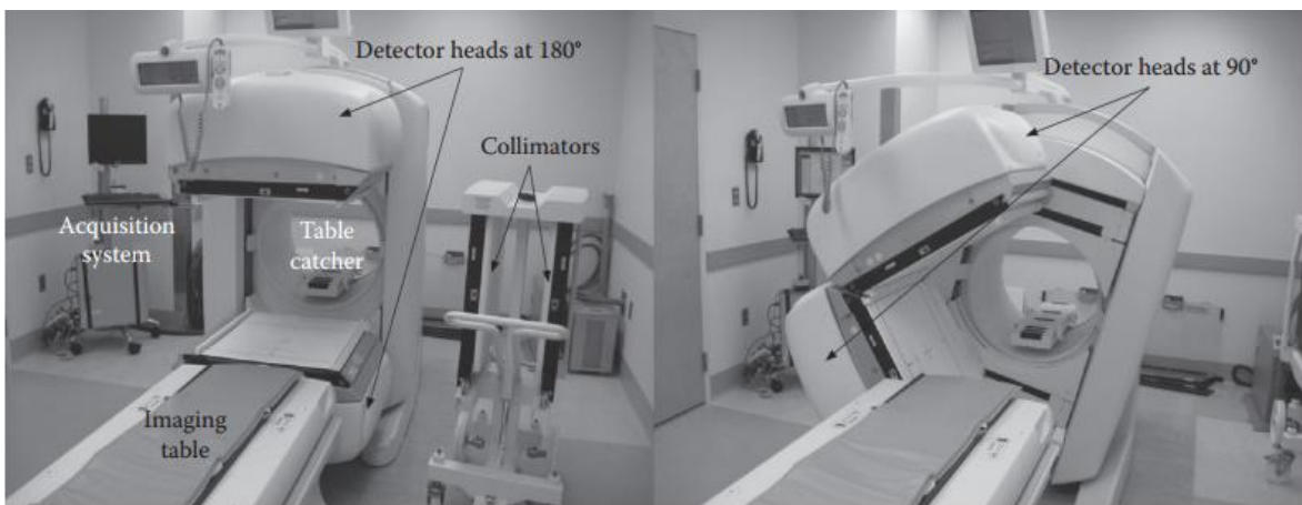
Figure 2-5: Modern two-headed SPECT systems shown in two different configurations of the detector heads ( 180^\circ to the left and 90^\circ to the right) [2].
