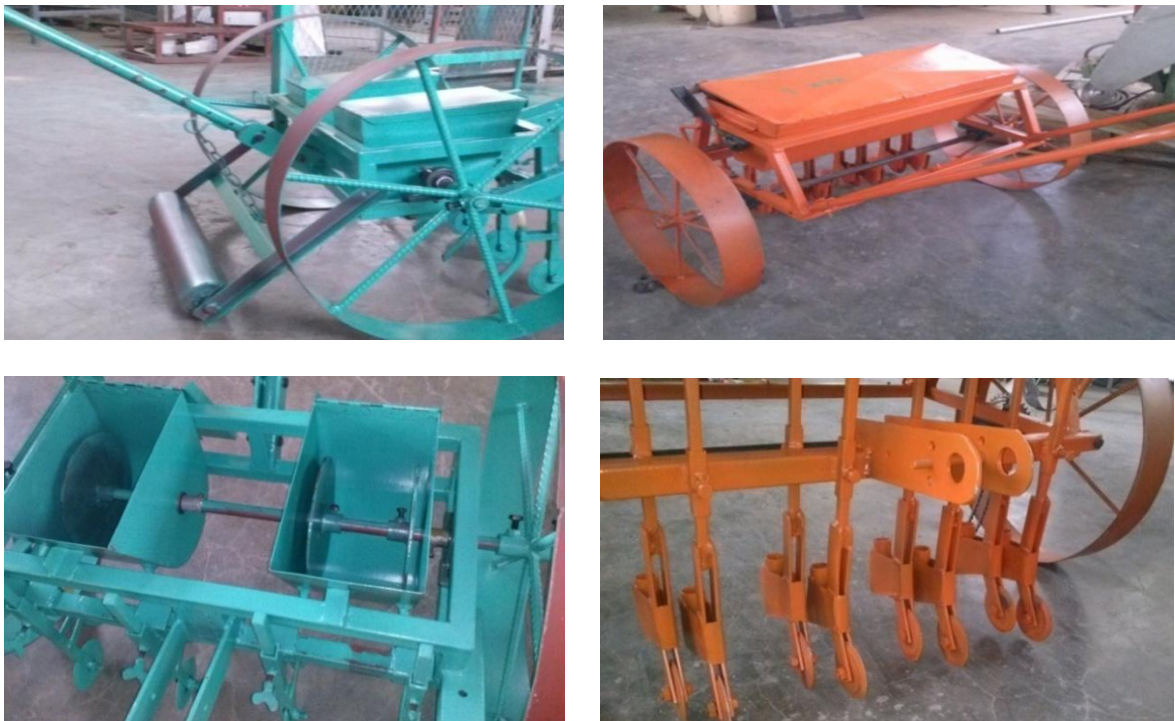
Figure 13: Teff Row seeder machine introduced by Ethiopian Institute of Agricultural Research (EIAR)
