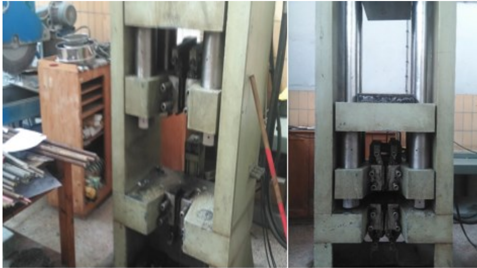
Figure 3-7: Steel reinforcement testing machine
