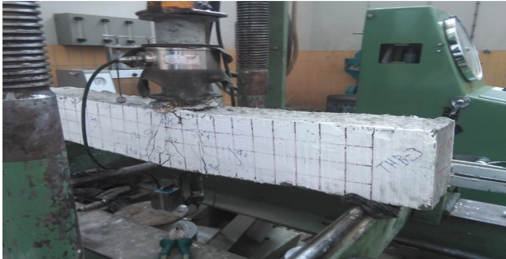
Figure 5-3: Experimental flexure failure crack patterns of THB-3
