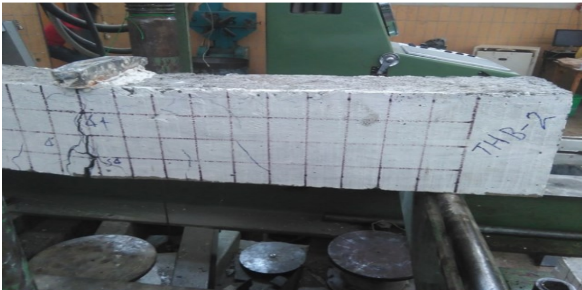
Figure 5-2: Experimental flexure failure crack patterns of THB-2
