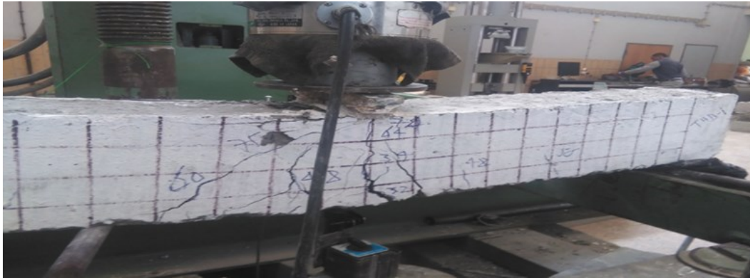
Figure 5-1: Experimental flexure failure crack patterns of THB-1
