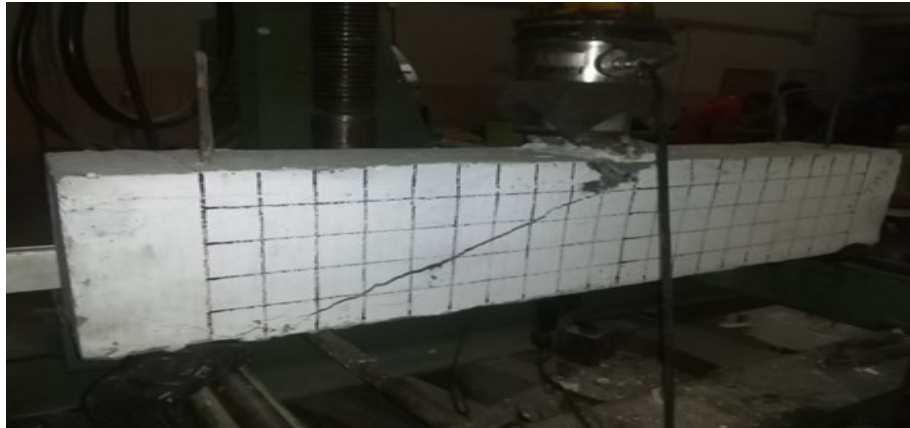
Figure 5-23: Experimental shear failure crack patterns of THB-6
