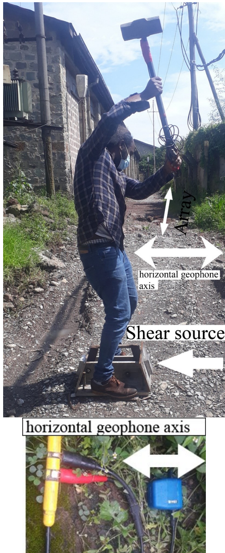
Figure 3-12: The typical set-up for shear-wave refraction acquisition.
