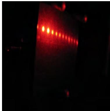
Figure 5.1: Diffraction fringe patterns before load applied
