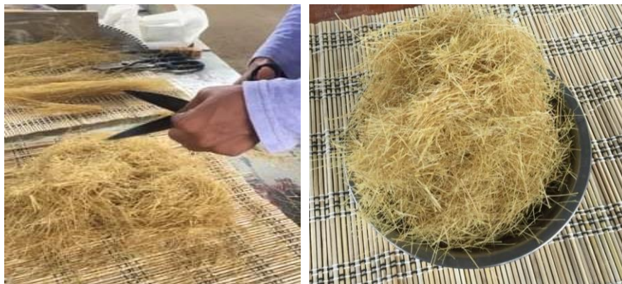
Figure 12 Fiber sizing process
