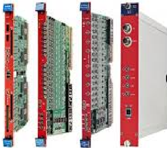
Figure 3.6: Modular detector electronics (High voltage supply, preamplifier, amplifier and multichannel analyser)
