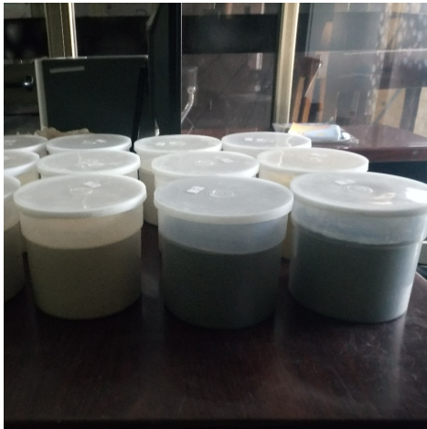
(c) Prepared samples for HPGe detector
