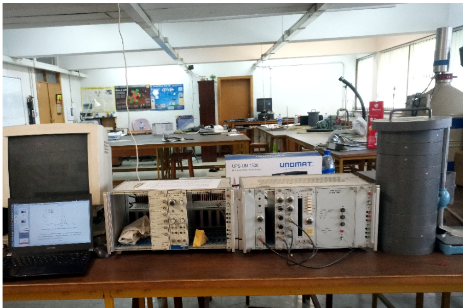
Figure 3.19: Gamma spectrometer with FJ374 scintillation crystal and Electronic circuits
