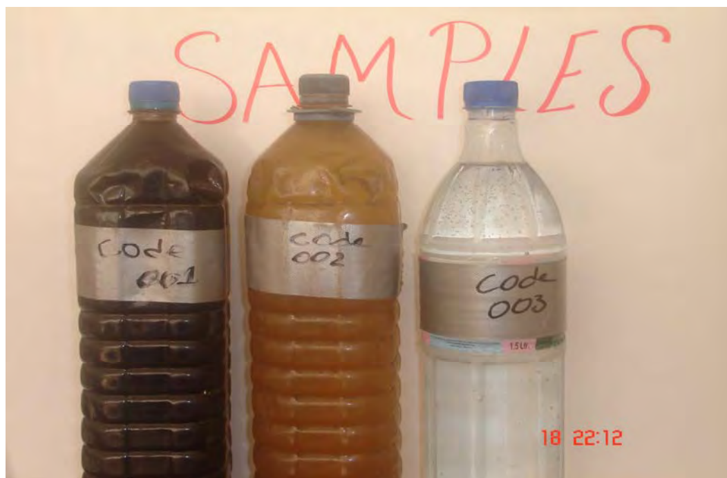
Figure 4.1: Samples collected for laboratory analysis from leachate, nearby well and spring water (from left to right).
