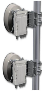
FIGURE 2.8: 4x4 LOS-MIMO direct mount configuration [4]
