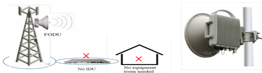
FIGURE 2.2: All outdoor microwave equipment
