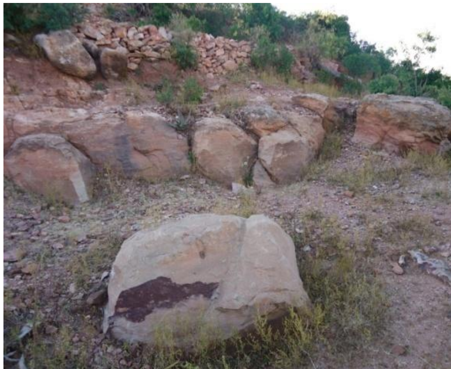
Figure 3.20 A recent grind stone quarry site within the large Maisheho quarry site with large syenite-phonolite blank rock for grind stone. This quarry site has dimensions approximately 8m width X 15m length.
