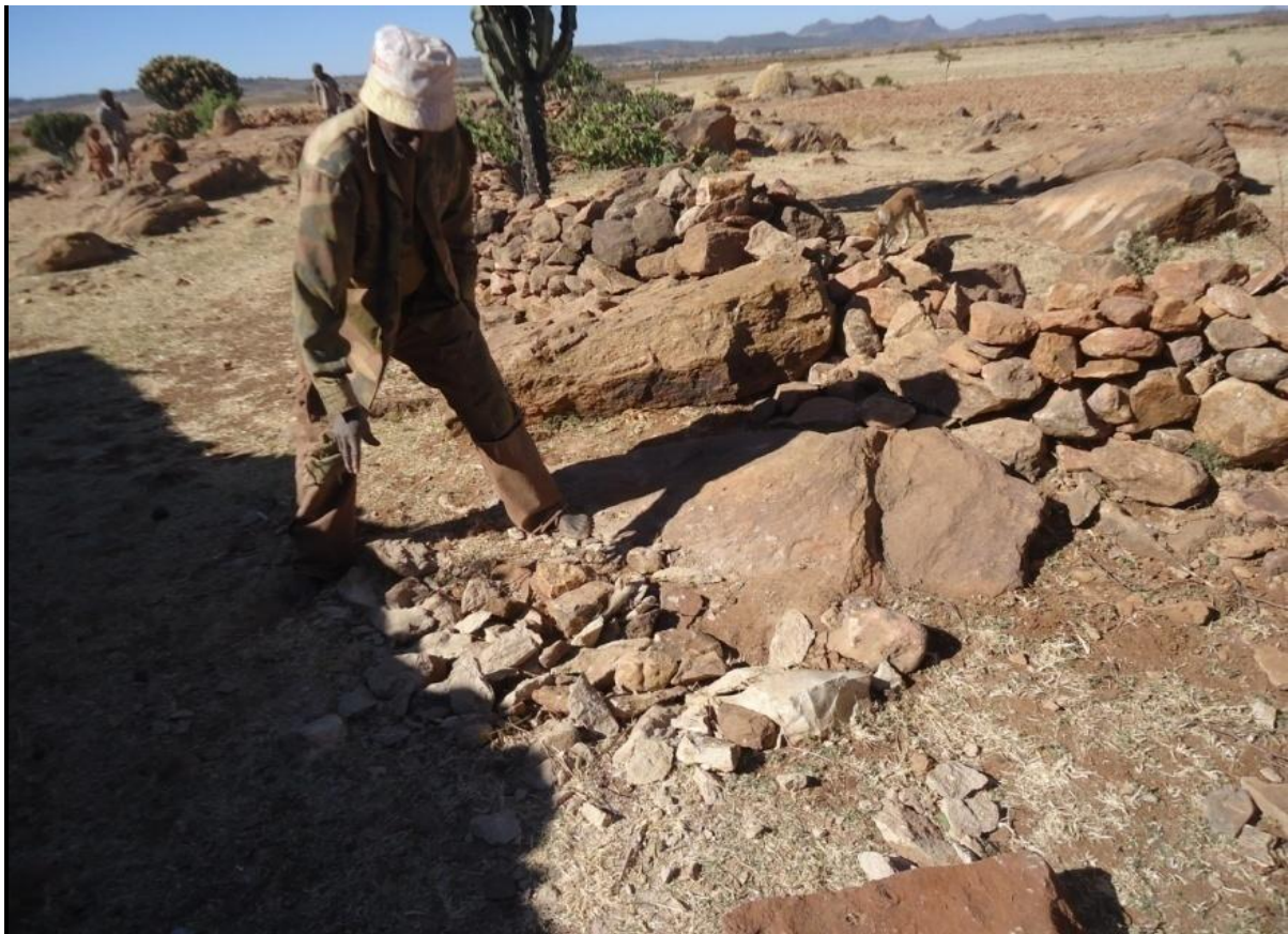
Figure 3.14 A quarry man (in Debresina quarry site) is showing to the researcher the refilled pit with chipped stones and flakes after the blank was acquired. Note that it was done so in order to avoid the possible danger of the pit up on domestic animals and humans while walking through it.
