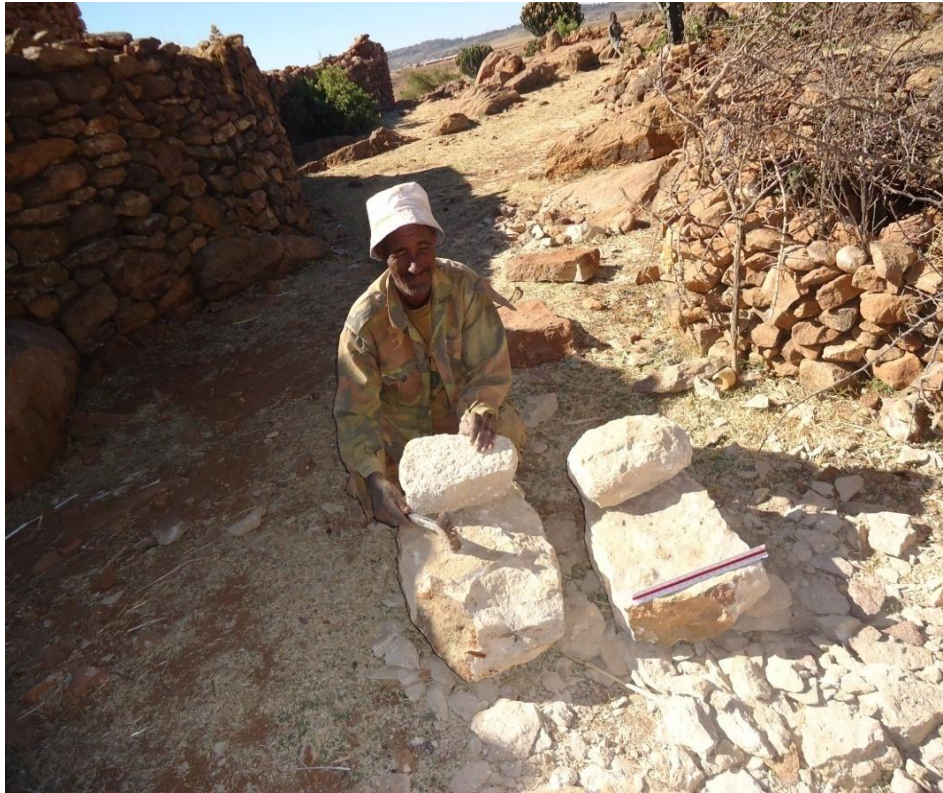
Figure 4.1 A quarry man shaping grind stones and manos using small hammer in Debresina quarry site. The flaked stones scattered around the semi finished grinding equipments were trimmed off deliberately by the quarry man.
