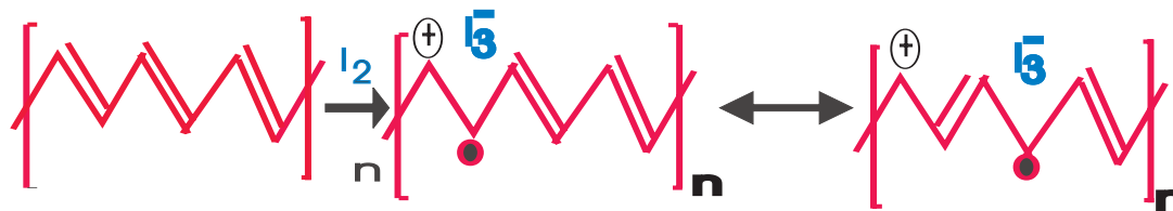
Figure 3.9: Doping of Polyacetylene gives polaron
