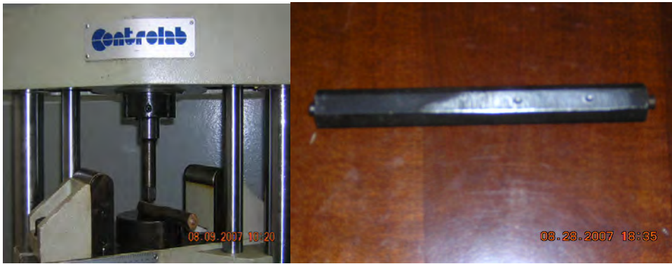
Figure 5.3 Nut sample being tested and after testing
