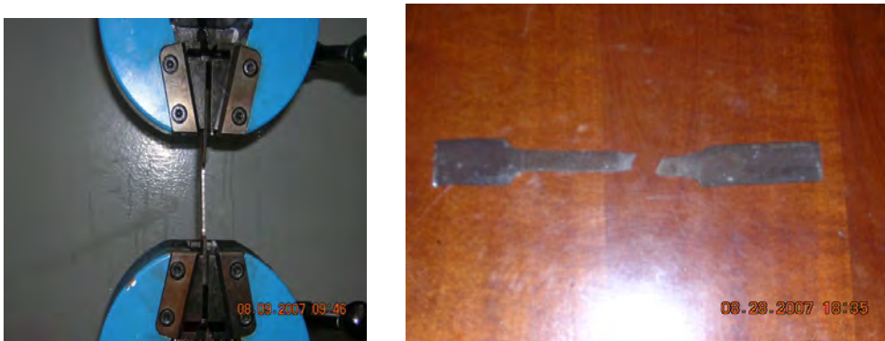
Figure 5.4 Struts sample being tested and after testing
