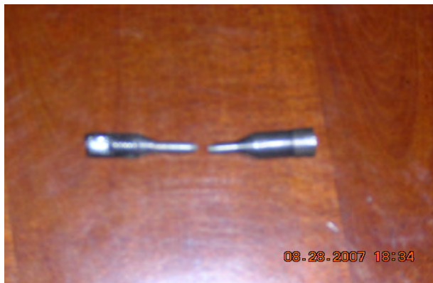
Figure 5.1 Bolt sample after testing
