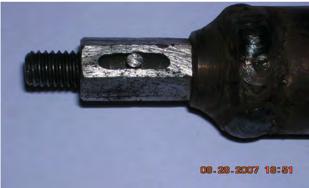
Figure 5.5 Connected bolt, nut, node and strut
