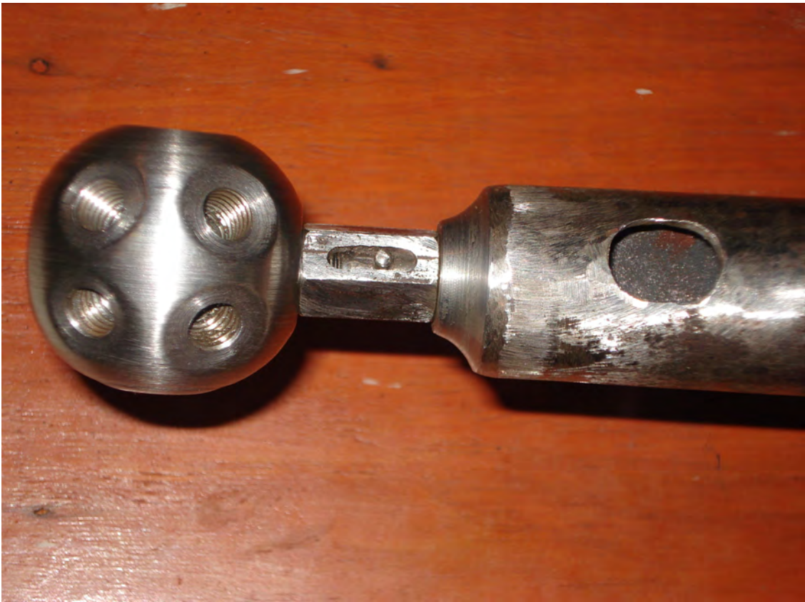
Figure 5.5 Connected bolt, nut, node and strut
