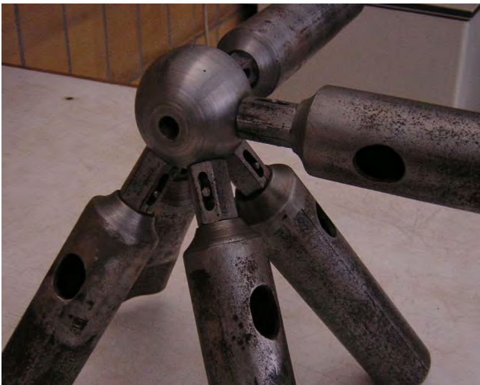
Figure 4.2 Struts to node connections
