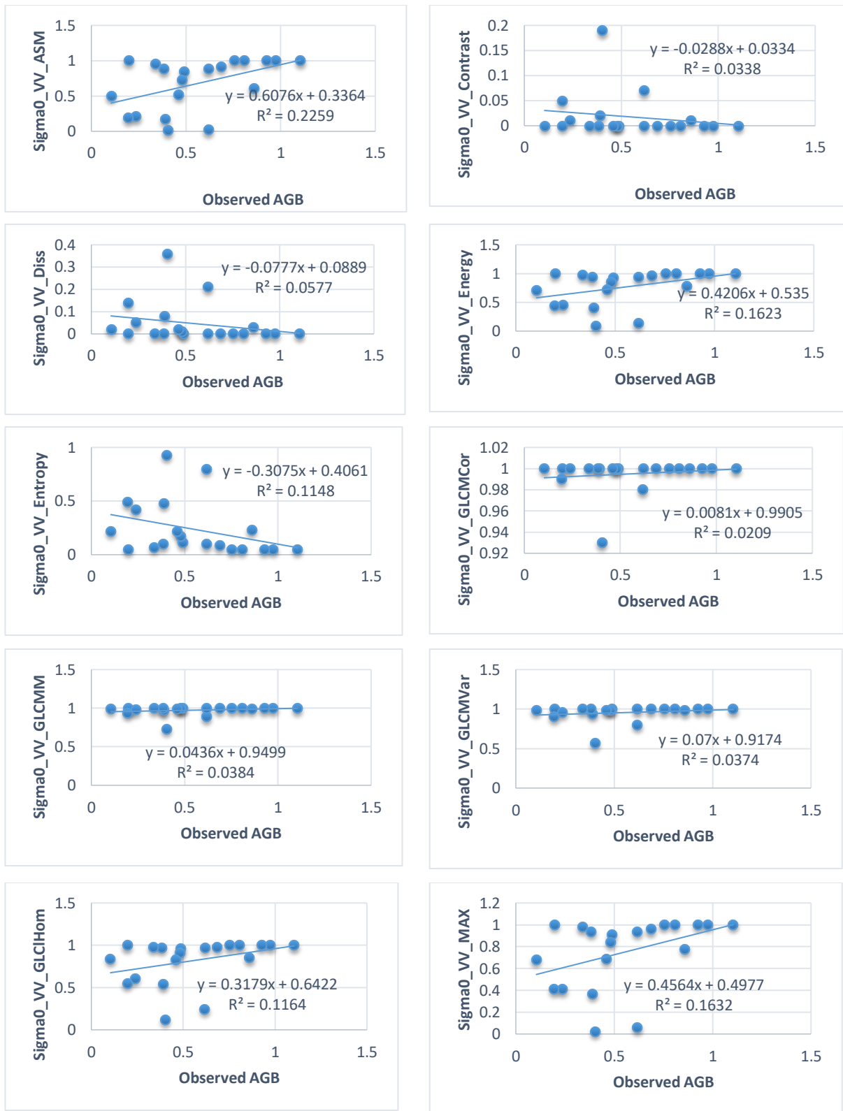
Figure 4.3: Scatter plot showing linear relationship between variables extracted from texture analysis of Sigma0_VV using grey level co-occurrence matrix and Observed AGB
