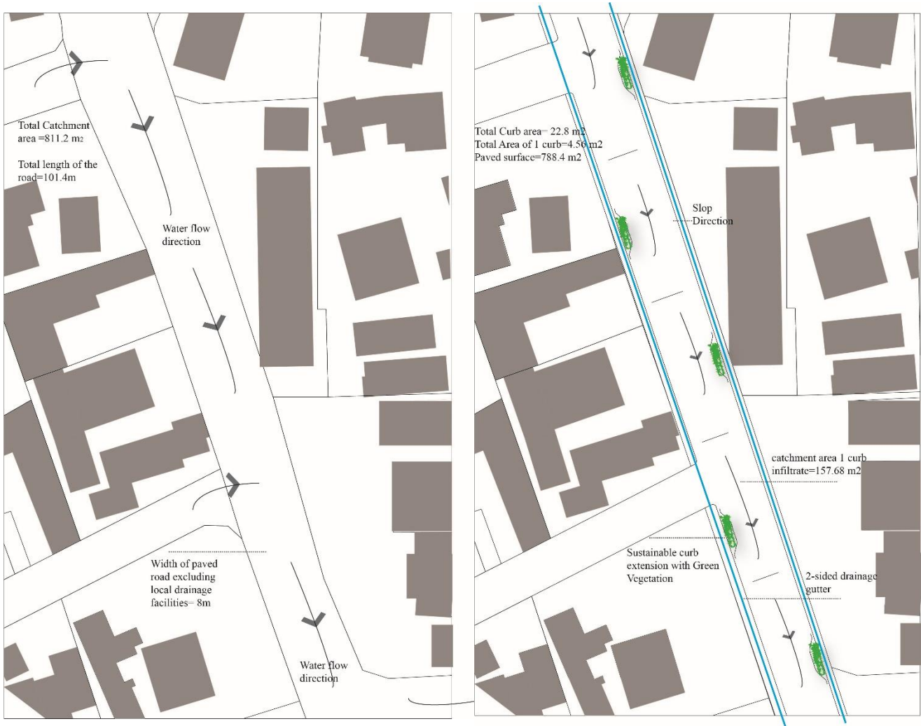
Figure 40: Existing case area (left side map) and study area plan with curb extension,(right side) drainage facility, individual and total catchment area of the curb infiltration capacity.
