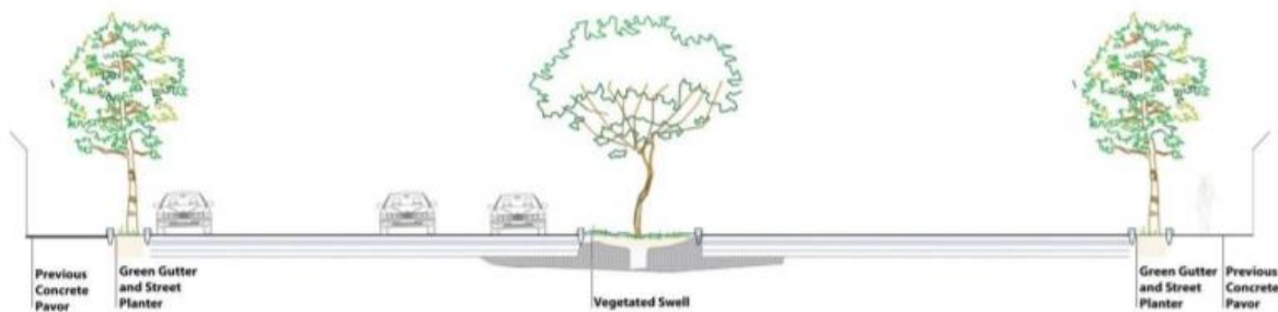
Figure 13: Green gutter and street planter (Source Liu, 2013).
