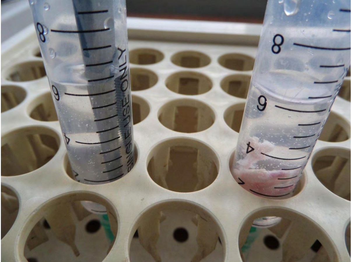
Figure 10. Forelimb and hindlimb muscle and bone volume measurement in a water filled syringe
