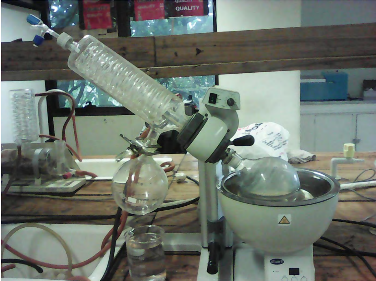
Figure 4. Adjusting concentration of hot water fish extracts by using rotary evaporator
