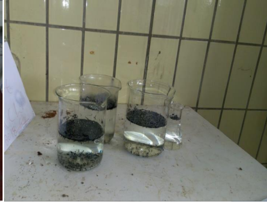
B.8: Hydrophobicity using water emersion test
