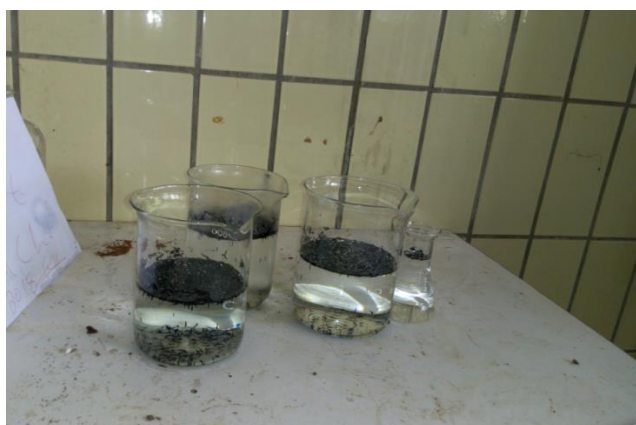
Figure 4.11: Hydrophobicity properties of torified rice husk using water emersion test
