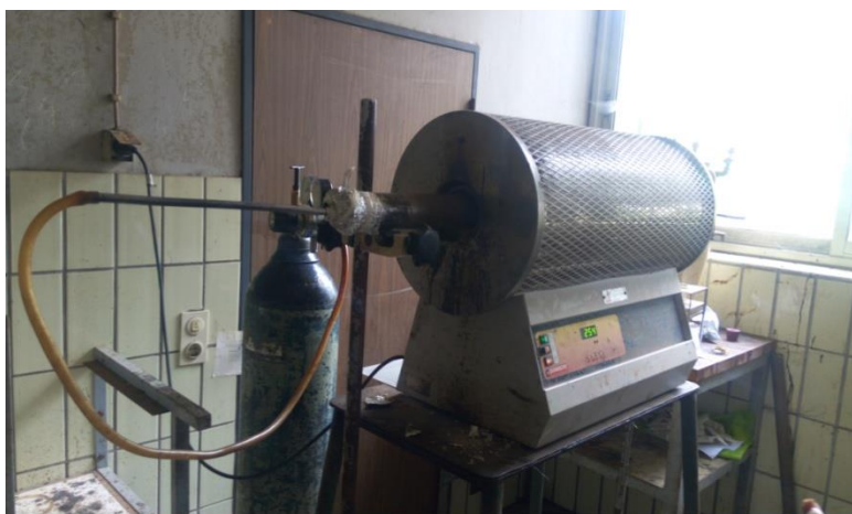
Figure 3.5 The experimental set up for the torrefaction experiments
