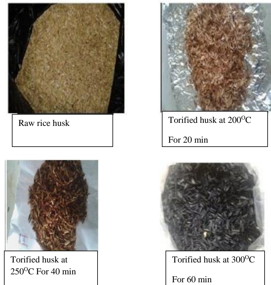
Figure 4.1: Effect of Torrefaction temperature on surface morphology of rice husk sample.
