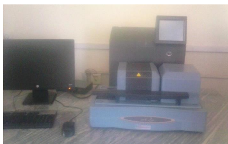
Figure 3.3: Thermo gravimetric Analyzer (TGA)
