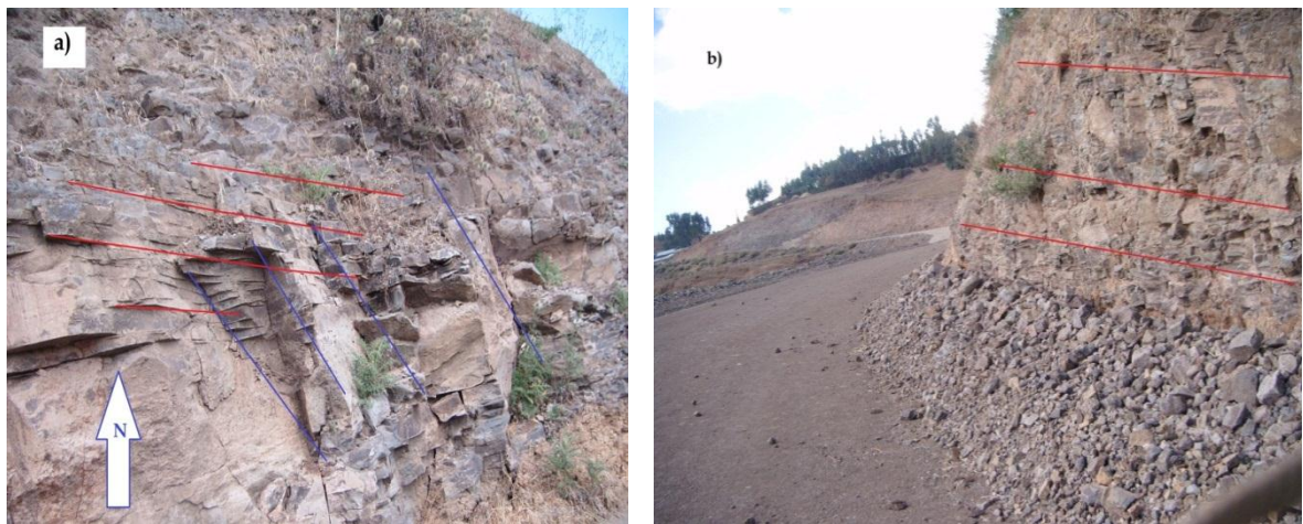
Plate: 3.3 a) two joint sets of ignimbrite. b) Horizontal lineaments on basalt.
