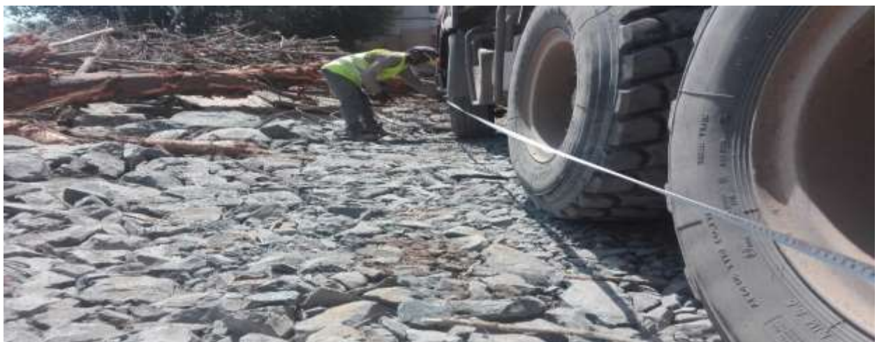
Figure 4.2 Measured axle load and spacing of Sino truck
