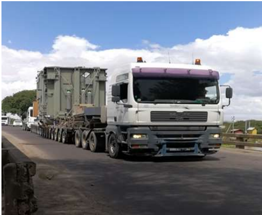
Figure 3.7 Heavy truck with multiple axle load carrying 172-ton transformer approaches and passes the bridge with a crawling speed of 4Kmh.
