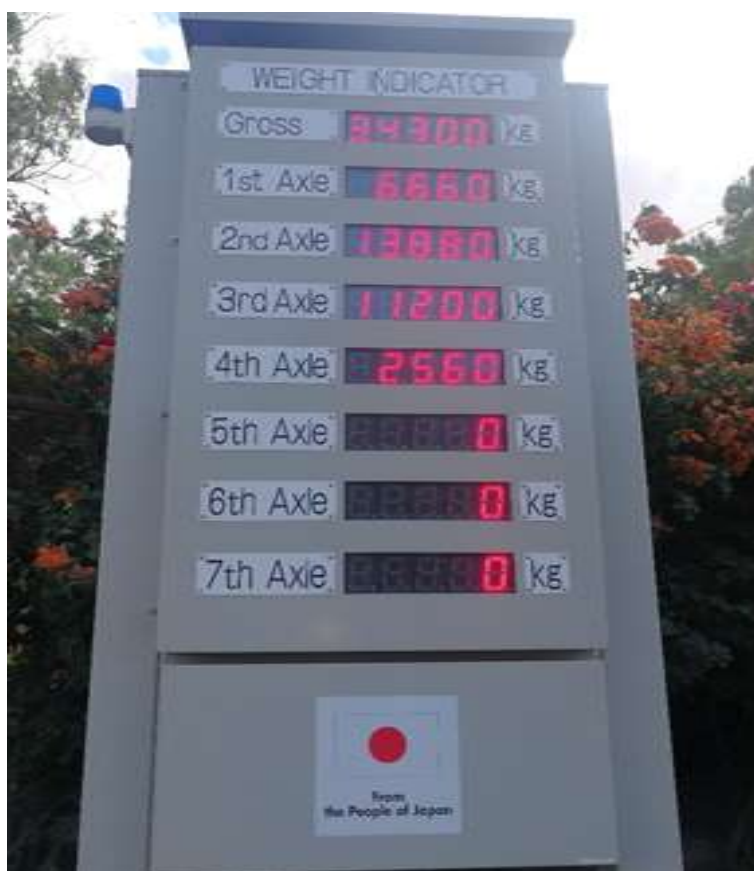
Figure 3.9 Measured axle weight of Sino truck from weighing station.
