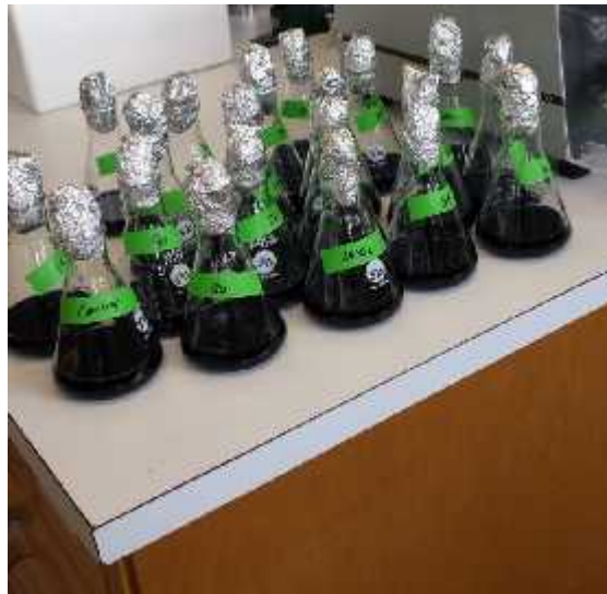
Phosphate solubilization on Tri-calcium phosphate, aluminum phosphate and ferrous phosphate in liquid medium
