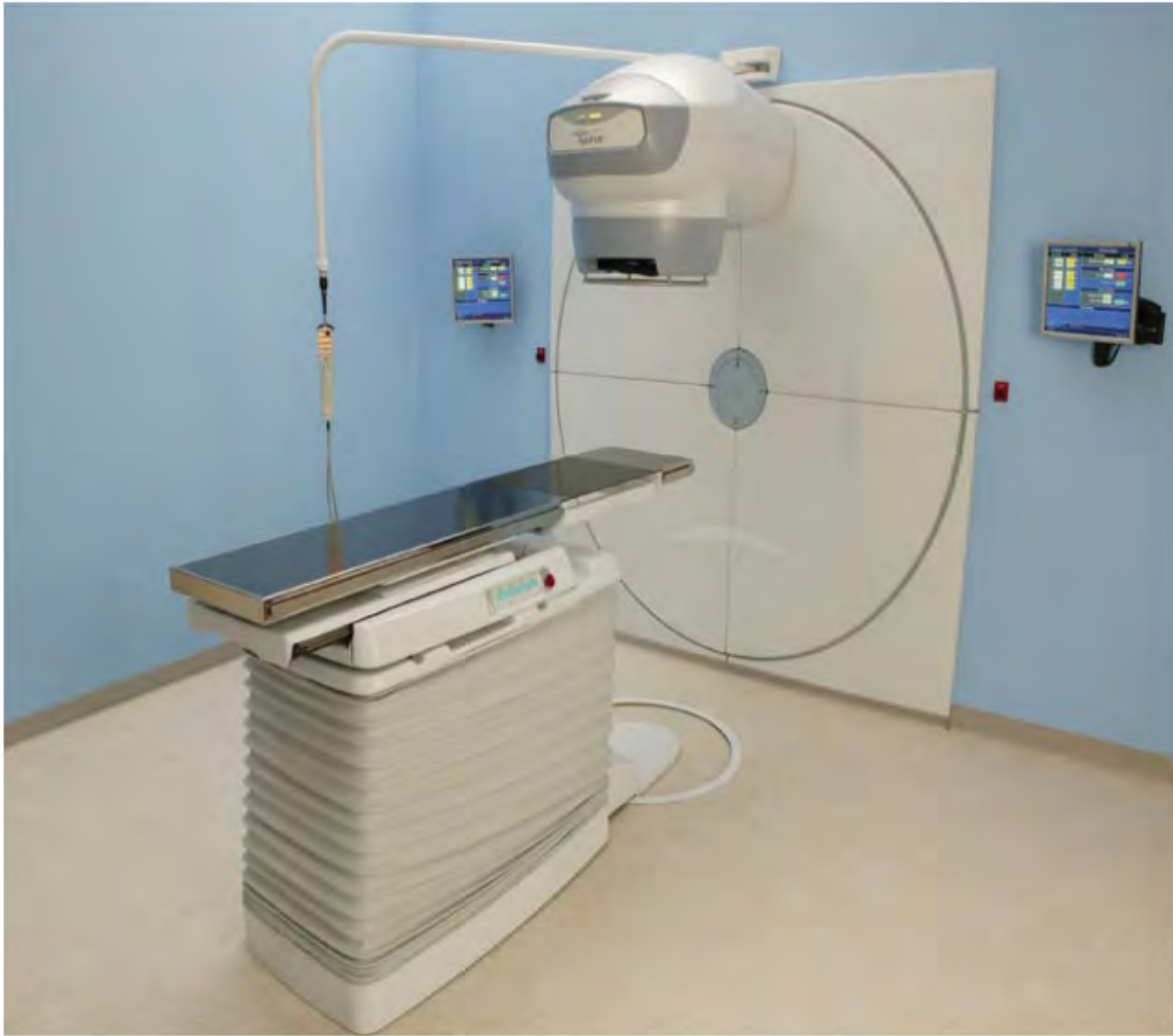
Figure 3.1: The picture of “Theratron equinox 80 ” 60 Co radiotherapy unit.
