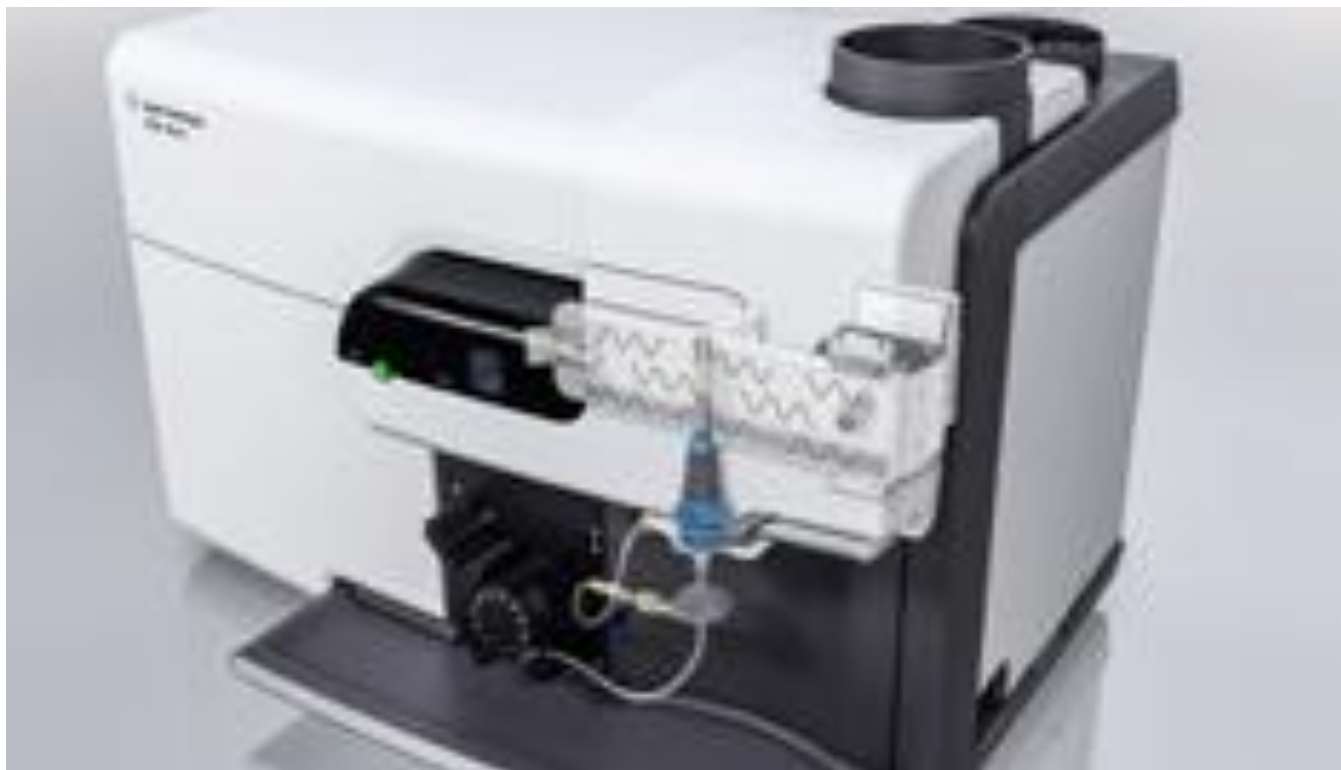
Fig.6: Schematic diagram of a microwave plasma atomic emission spectrometer
