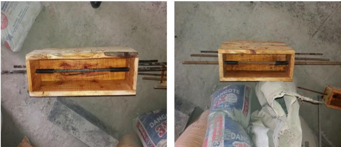
Figure 3-1 Unbonded length of bar by PVC
