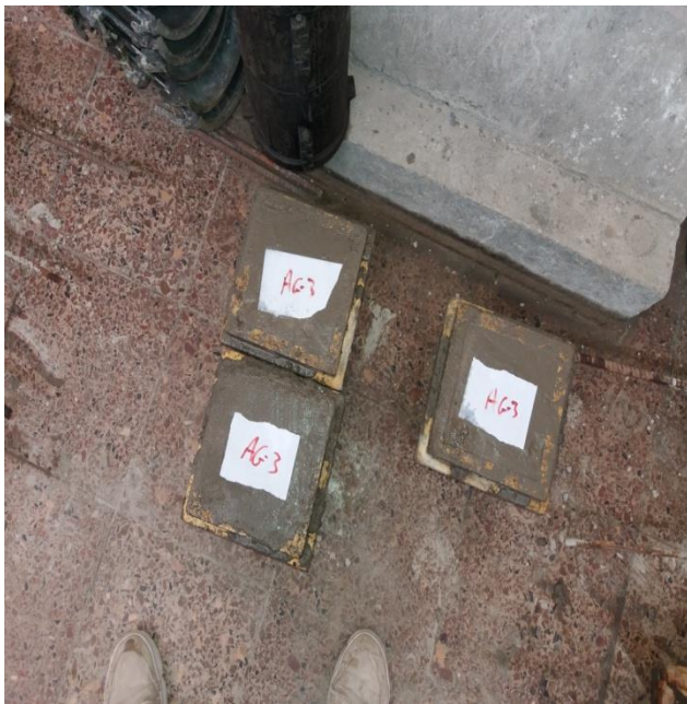
Figure 3-2 cubes for trial mix
