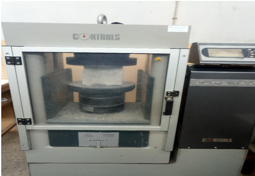
Figure 3-4 Compressive and tensile strength testing machine for concrete
