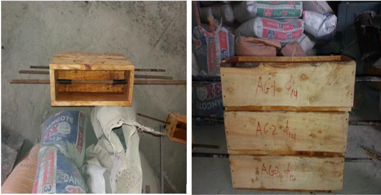
Figure 3-6 prepared mold for casting concrete
