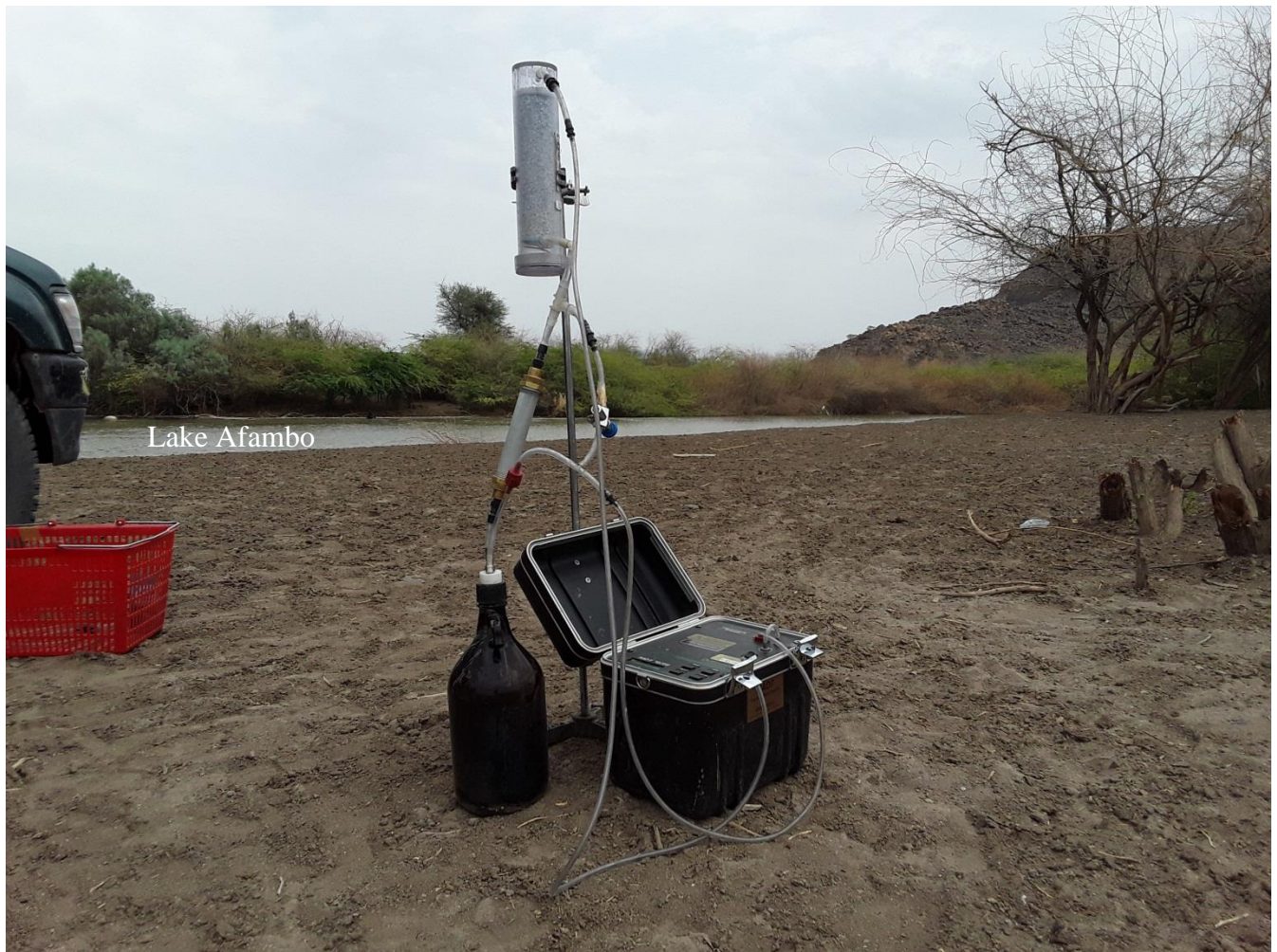
Figure1.1 On site Radon measurement
