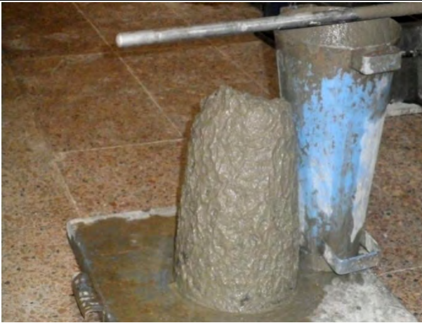
Slump test of C-40, OPC
