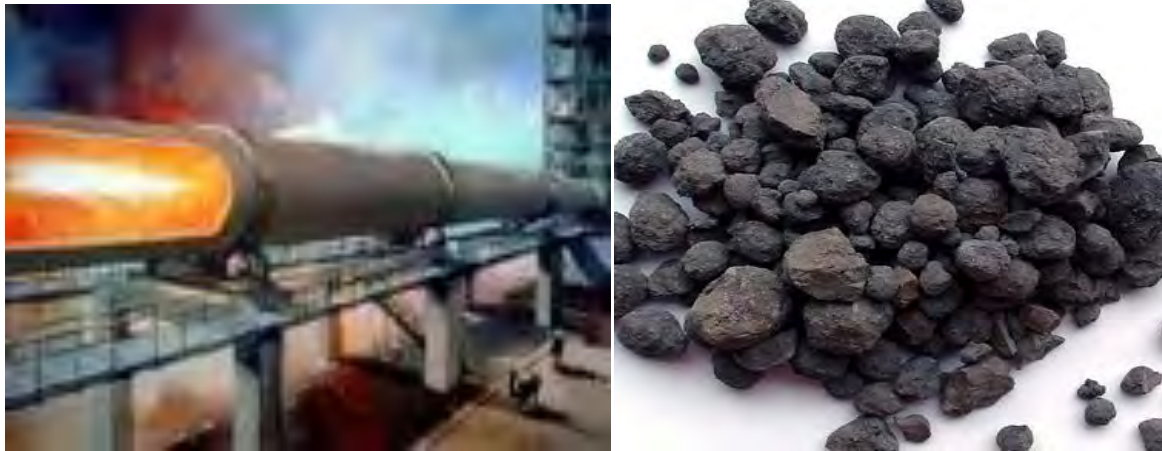
Fig 2.3: Burning the mixture in the kiln and formation of Clinker [24]
