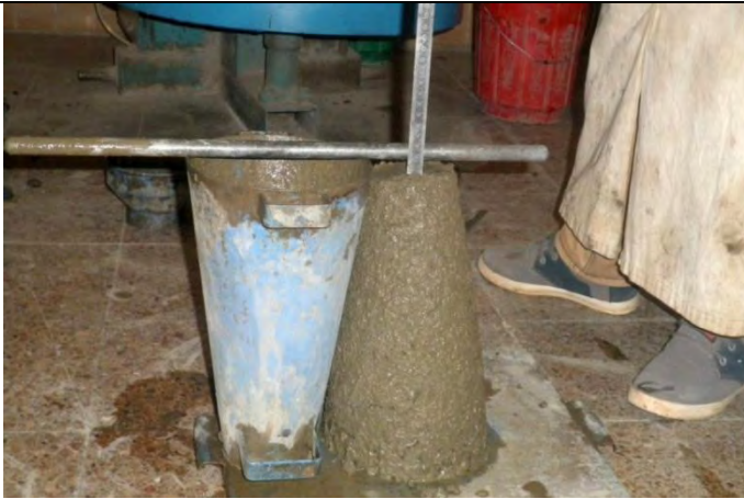
Slump test of C-90 & C-100 from OPC and C-70 from PPC
