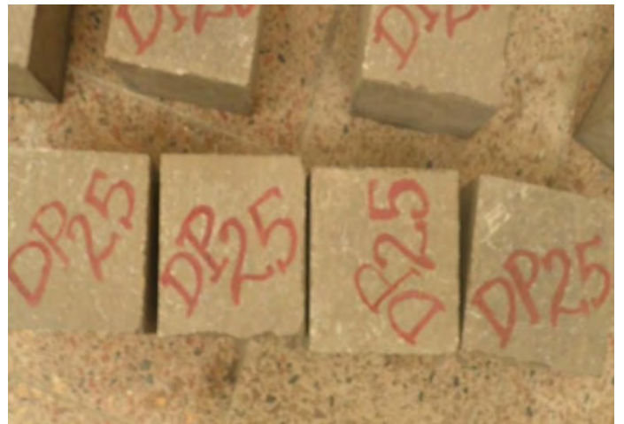
Batch of C-25 concretes, PPC (after removing the molds)
