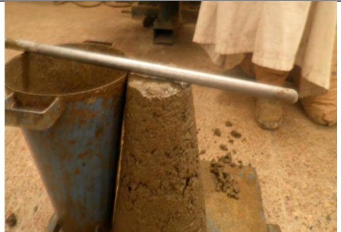
Batch of C-25 concretes, PPC (after removing the molds)
