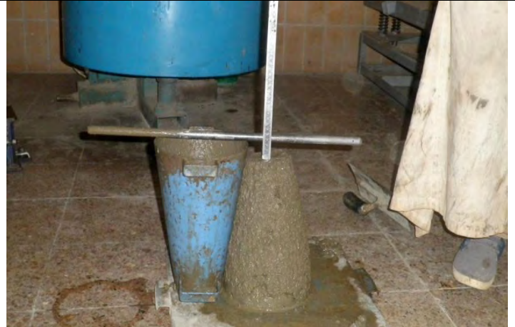
Slump test of C-60, OPC
