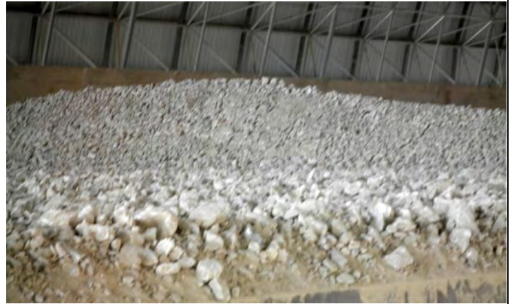
Sand Stone, ready for proportioning
