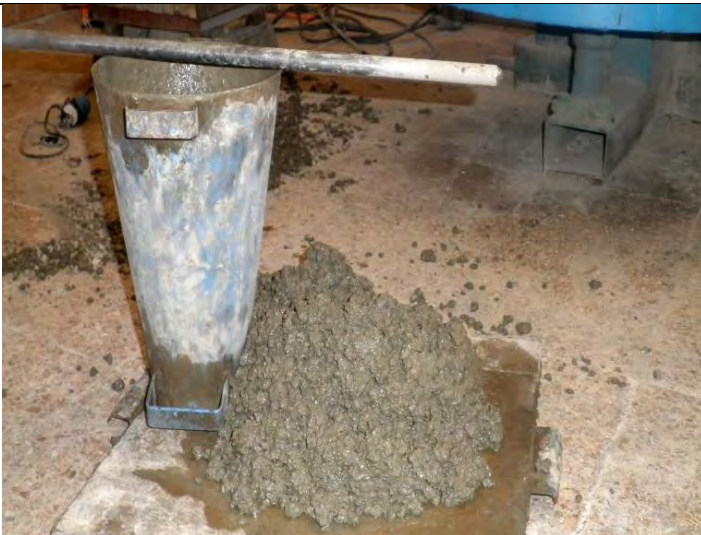
Slump test of C-90 & C-100 from OPC and C-70 from PPC
