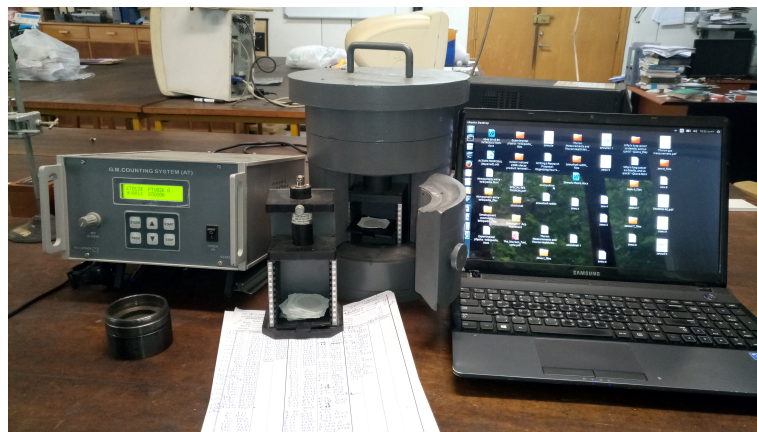
Figure 3.4: The GM Counting System at the nuclear and radiation physics lab, AAU
