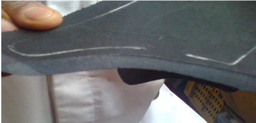
Re-enforcing the leather component using textile fabrics
