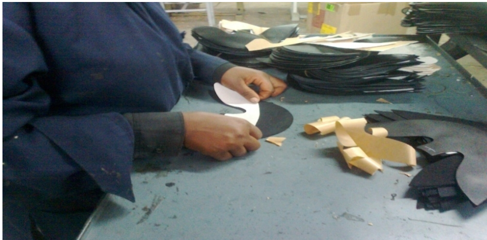
Re-enforcing the leather component using textile fabrics
