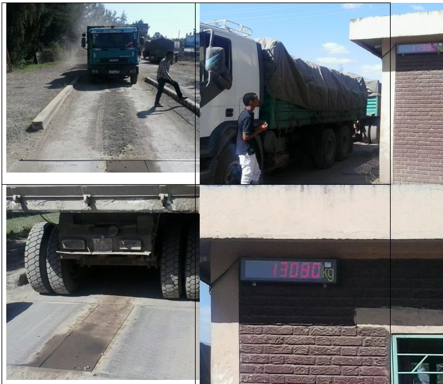
Figure 4-2: Axle load measurement at Holeta weighbridge
