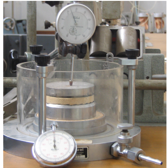
b) consolidometer without loading bar
