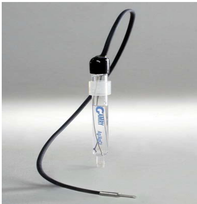
Figure 8 A typical silver-silver chloride reference electrode
