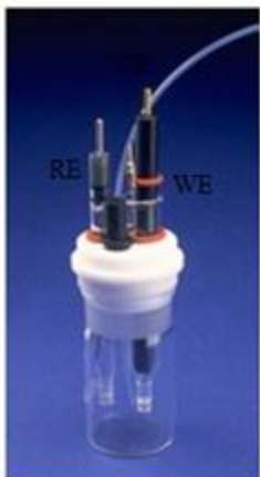
Figure 11 Setup of an electrochemical cell
