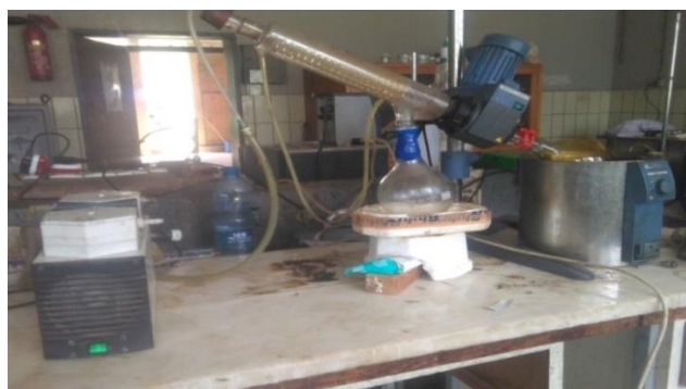
Figure 7: rotary evaporator under vacuum
