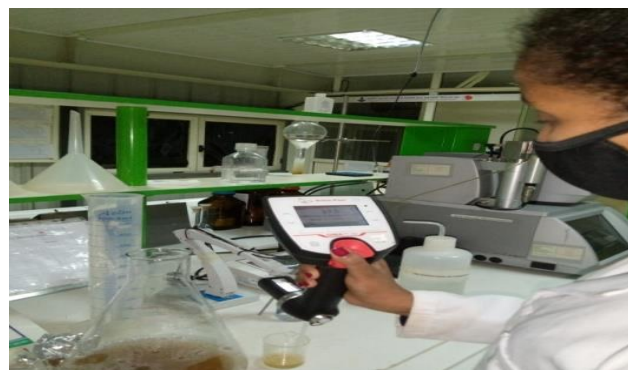
Figure 15: Density meter analysis (DMA 35)
