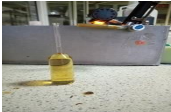
Figure 19: density measuring pycnometer
