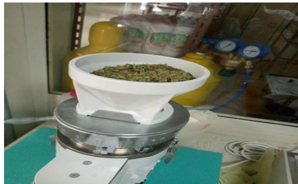
Figure 5: Disc mill DLFU Buhler
