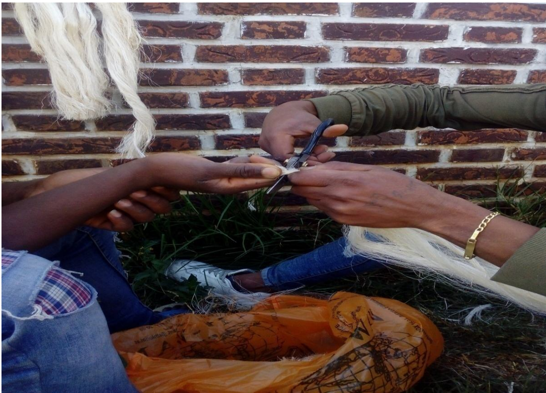
Figure 3. 3 Manual chopping of enset fiber into smaller pieces
