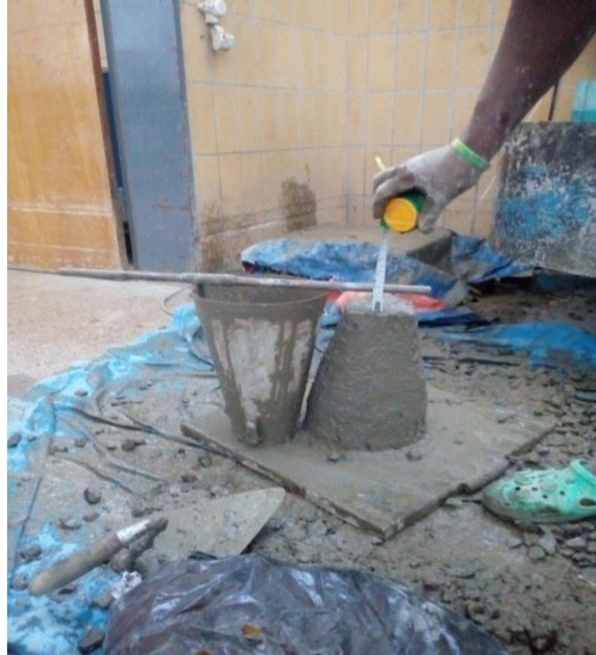
Figure 3.6 Workability Test Using Slump
