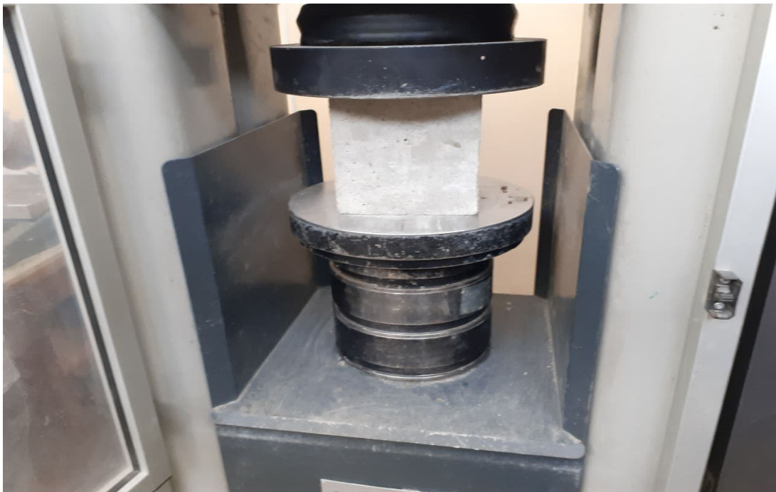
Figure 3. 7 Compressive strength testing
