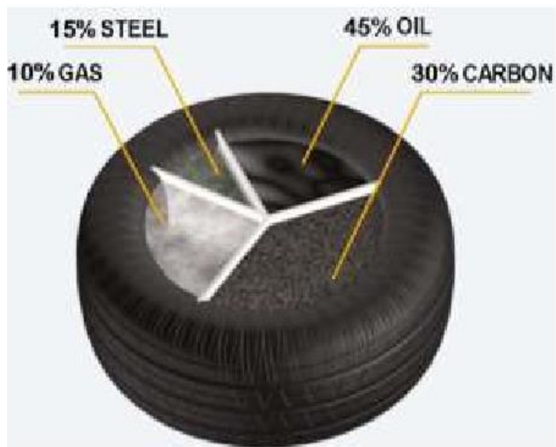
Figure 2.20 Products % after recycling by pyrolysis
