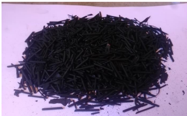
Figure 3.1 Sample ready to ash and moisture content measurement
