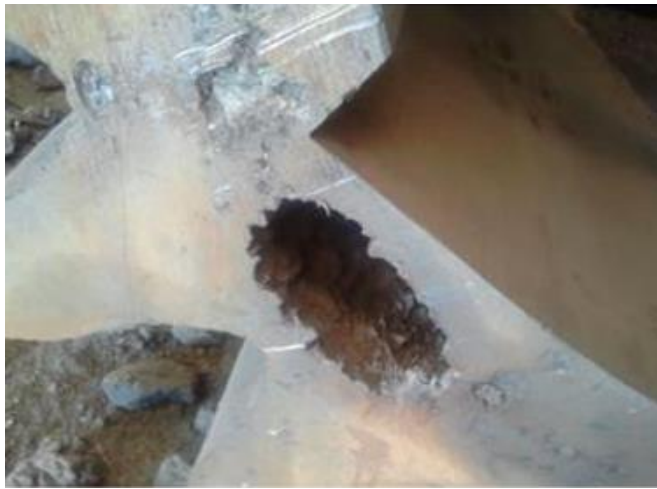
(e) Shrinkage cavity and Sand sintering
