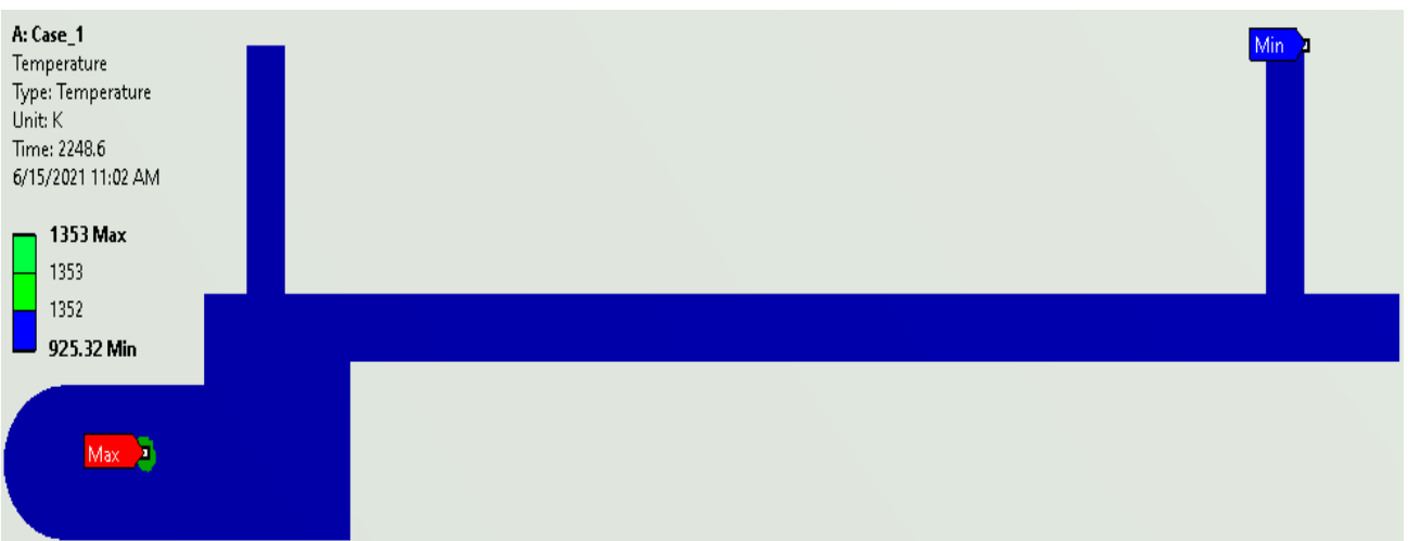
(c) 2248.6 seconds (solidification ends)
