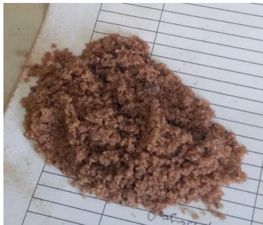
Figure 3.2- Sample silica sand bonded with risen The machine has five-digit readability. To determine the specific gravity of the silica sand, a 50 \text{ cm}^3 specification pycnometer used to put the silica sand.
