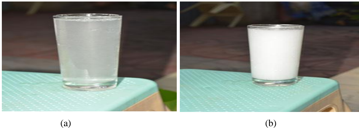
Figure 3. 6: (a) is contaminated water with 100mg of sodium nitrate and (b) is contaminated water with 400mg of sodium nitrate.
