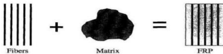
Figure 5: Formation of Fiber Reinforced Polymer Composite
