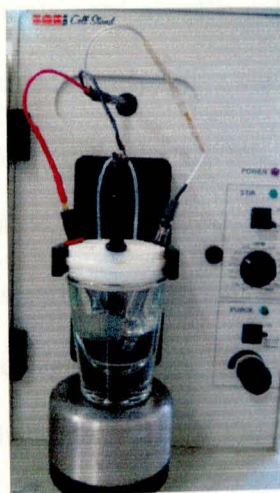
Figure 3.1. Electrochemical cell consisting of working electrode (black), counter electrode (red) and reference electrode (white)
