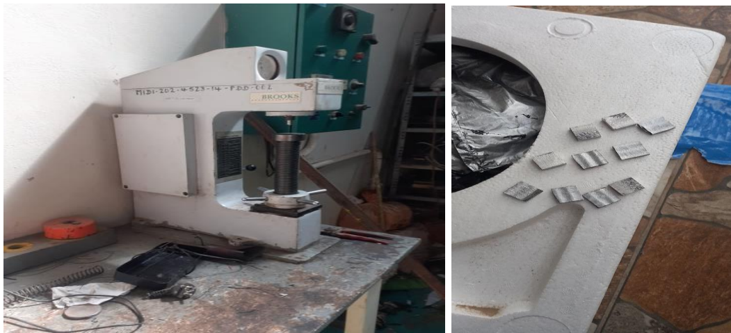
Figure 3.11 Rockwell hardness test specimen test on the machine and specimen after test
