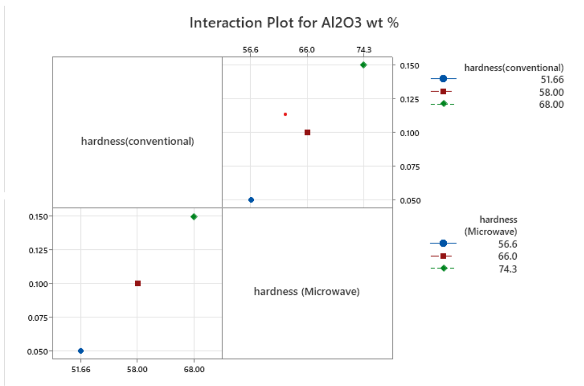
Figure 4.17 Interacting effect of Rockwell hardness test with heat treatment and \text{Al}_2\text{O}_3 content
