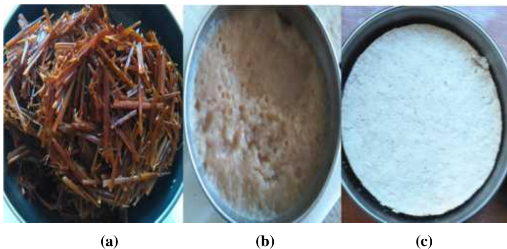
Figure 10 Pulp from digester (a), after washing (b), after drying in an oven(c)
