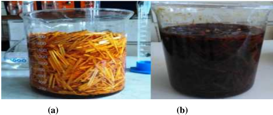
Figure 9 wheat straw before cooking (a) after cooking (b)
