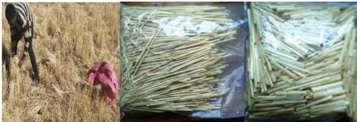
(a) (b) (c) Figure 7 Wheat straw while harvesting (a) after dried (b) and size reduced (c)
